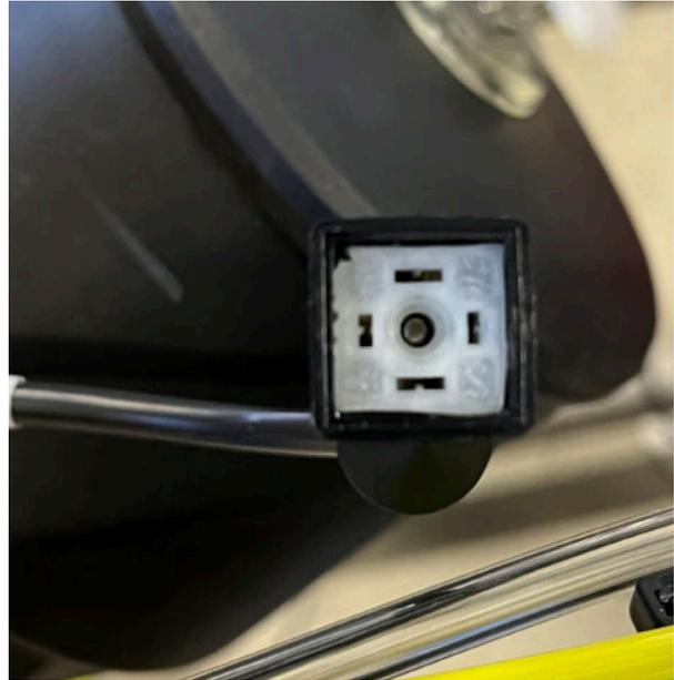
**Fig. 7.2.1 - 2** - Pressure transducer (left) and DIN cable connection (right)
