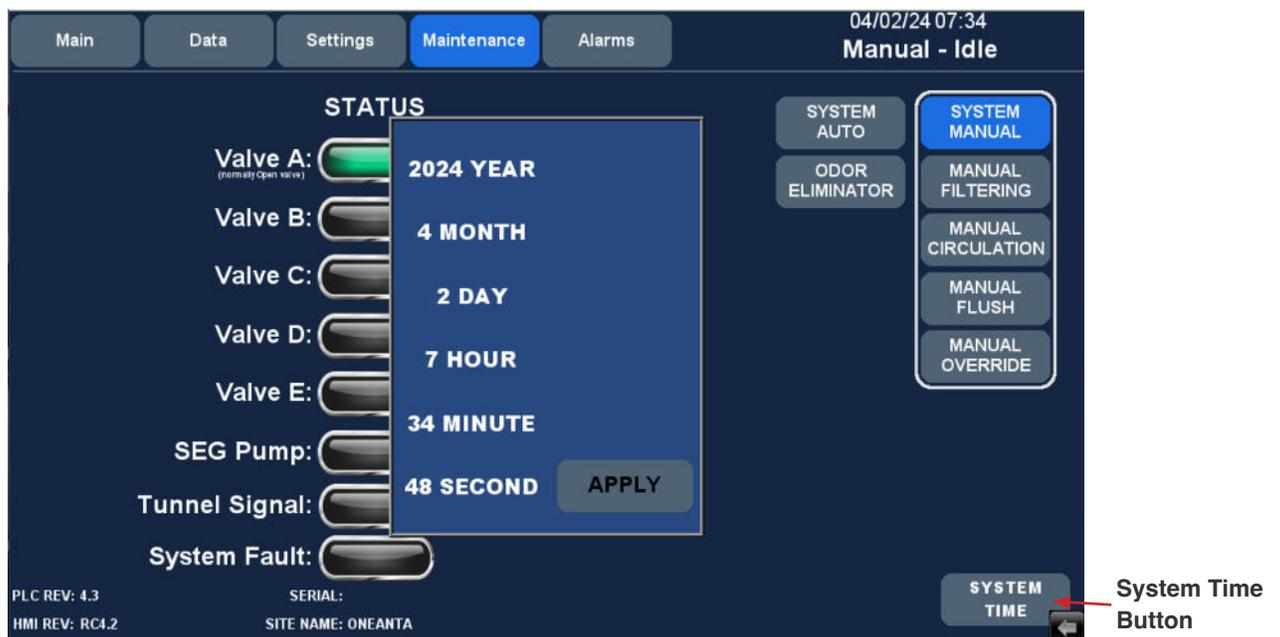
Fig. 6.1 - 1 - Resetting HMI clock
