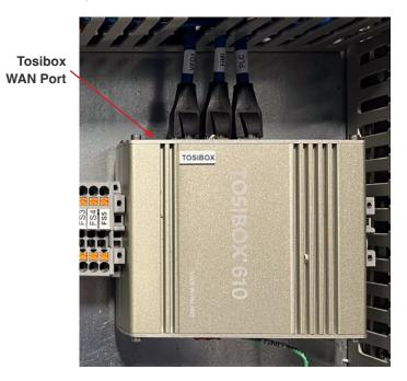
Fig. 3.3.2 - 1 - Tosibox WAN port connection for remote support
