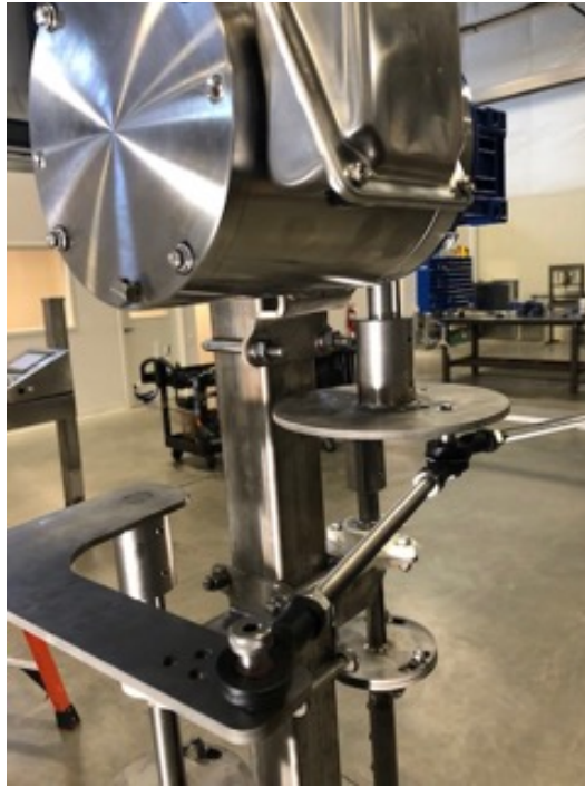
Fig. 3.2.2 - 1 - Flywheel/pitman arm connection
