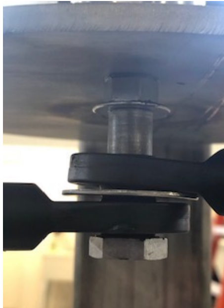
Fig. 3.2.2 - 2 - Installation of 2 linkages on 1 shoulder bolt
