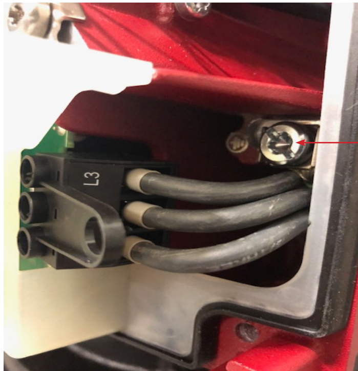
Fig. 3.3 - 2 - Pump grounding conductor and ground lug
