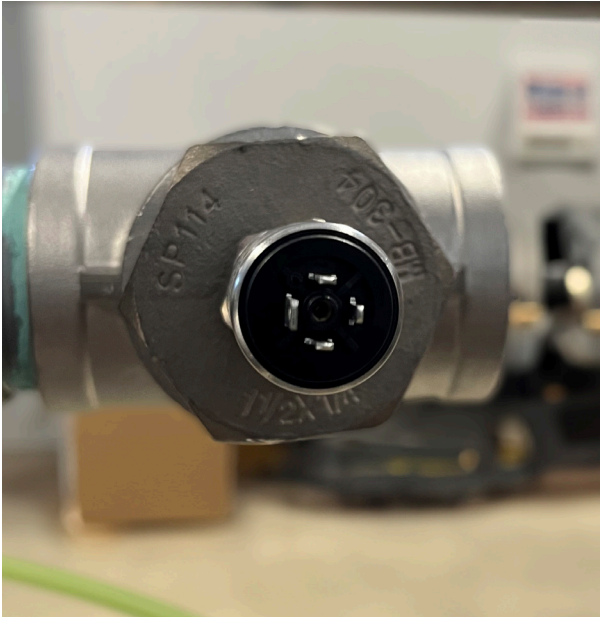
Fig. 7.2 - 2 - Pressure transducer (left) and DIN cable connection (right)
